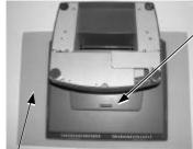
Press the Lock/Release button and slide the stand assembly downward (as viewed from the main unit) to detach it from the main unit.
